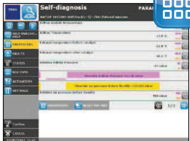
PARAMETER/STATUS screen showing the inputs and outputs managed by the ECU, displayed in numeric format and on graphs.
