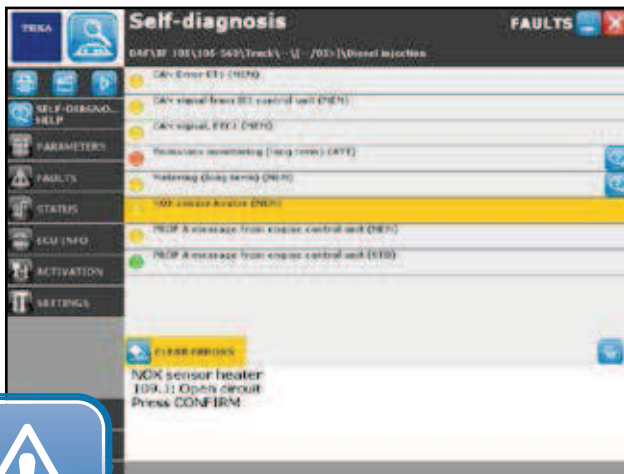
ERROR screen listing the faults/malfunctions saved in the ECU, with a detailed description of each one.
