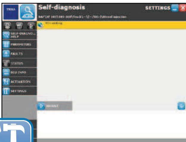
SETTINGS screen, offering the possibility to run the calibration, initialisation and programming functions required by the system, thus completing any repairs.
