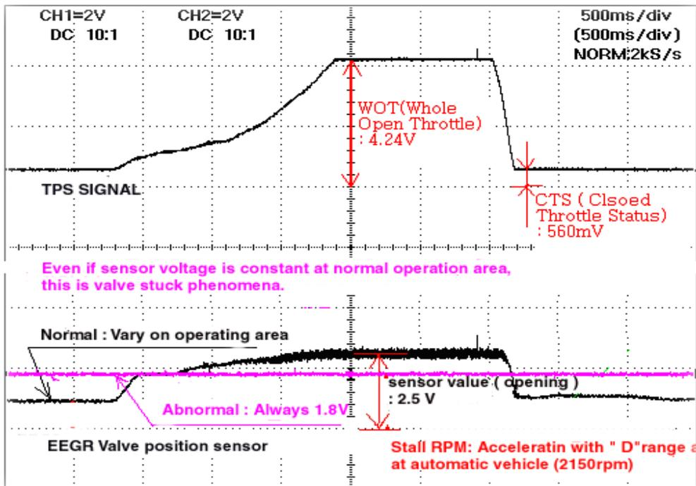
**Explanation** : EGR valve stuck is often occurred. U.S export vehicle is equipped with temperature. If low temperature is maintained with EGR operating range, ECU recognizes closing stuck. In the contrary if high temperature is maintained with non-operating range, ECU recognize opening stuck.
