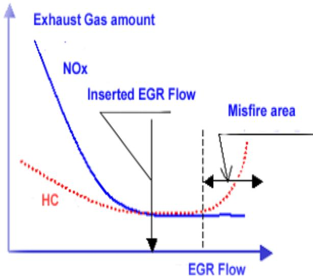
flame propagation. If it disturbs too much flame propagation, misfire will happen. Therefore valve opening is decided not to get misfire. In case of mechanical type EGR valve, valve opening is controlled by adjusting solenoid valve which is connected to surge tank to deliver under pressure to EGR, while Electrical type is directly control EGR valve opening.
