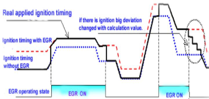
So, separate spark time is applied when EGR is operating. Then, how much does spark must be retarded with EGR?
