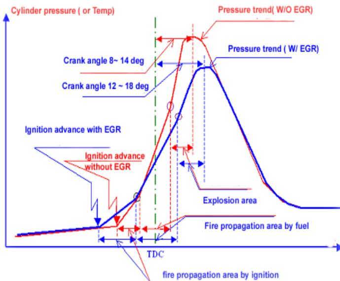
High combustion temperature ( it depends on compression ratio and air quantity but normally 1000 - 1400°C ) produce nitrous-oxide emissions( $\text{NO}$ ,  $\text{NO}_2$ ,  $\text{N}_2\text{O}_2$ ) by oxidizing the nitrogen( $\text{N}_2$ ) in the air. These nitrous-oxide emission is more produced with high temperature.
