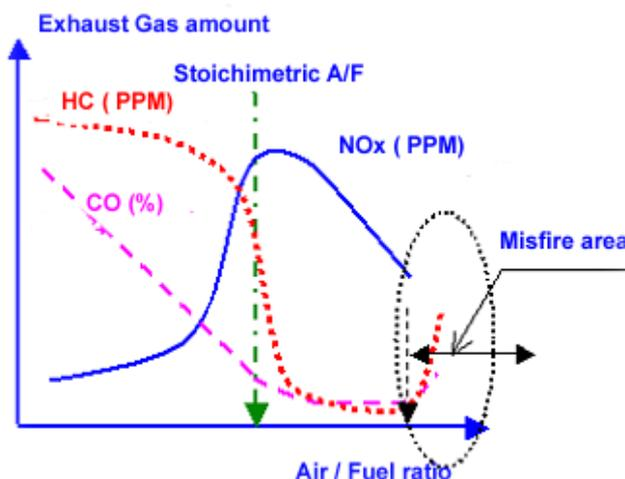
And nitrous-oxide emission is also depending on air fuel ratio and it is generated well with lean mixture (  $\lambda = 1.1$  ). So, nitrous-oxide emission should be considered seriously with current car, which uses stoichiometric air fuel ratio by oxygen sensor feedback control.
